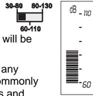
Normally, select the range in which the upper dB level is greater than any expected sound pressure level. The 60 to 110dB range is the most commonly used range. Use the 30 to 80dB range in quieter areas such as offices and classrooms.
